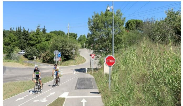
Example of how a Wattway Pack can power a security camera.
